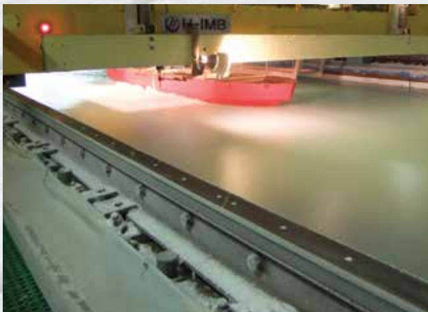
One of three hull forms tank-tested
